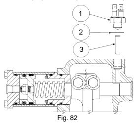
42. Check for continuity across the leads of the sensor with a continuity tester. The tester should indicate a closed circuit with air pressure applied to the air shift cylinder. See Fig 83.
