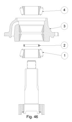
4. Install the end-float set-up tool or front output yoke and lock nut.
