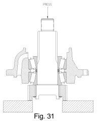
2. This completes the disassembly of the front output shaft assembly.
