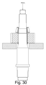
5. This completes the disassembly of the rear output shaft.
