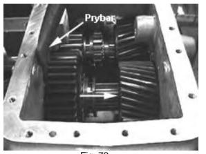
Fig. 72 29. Install the rear output yoke onto the shaft and torque to spec. See Fig. 73.
