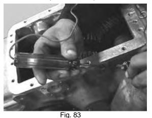
43. Install front output shaft into declutch housing using a new gasket. Align bearing oil drain with the bottom of the case. Apply Loctite #272 to bolt threads and torque to spec. See Fig. 84.
